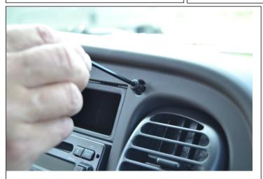
1. Remove the two screws above the upper right and left corners of the cubby or storage box in the upper center of the truck dash.
