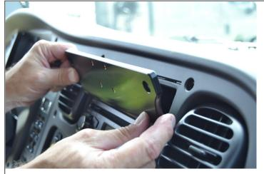
2. Insert the ProClip center mount into the space so the holes in the upper right and left corners of the center mount align with the holes where the screws were removed.
