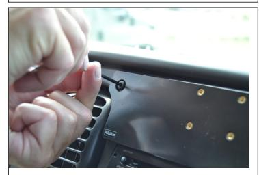
3. Reinsert the screws into the holes they were removed from and tighten the screws.
